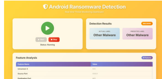
Fig. 7. Web interface displaying real-time prediction results with feature values.
